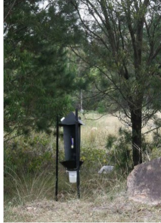
Static panel trap to detect Sirex wood wasp during flight season
