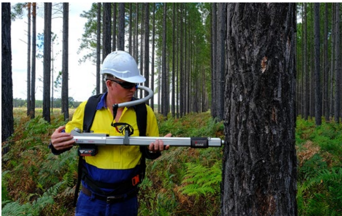
Using non destructive sampling tools to assess wood quality to support our marketing and genetic improvement strategies
